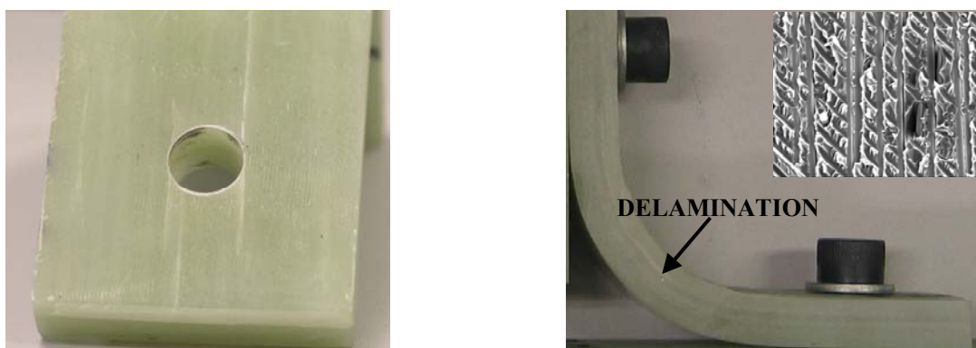
Figure 19: Damage induced in a bolted GRP T-joint resulting from direct tension loading. (left: longitudinal splitting around bolt hole; right: delamination in flange)
