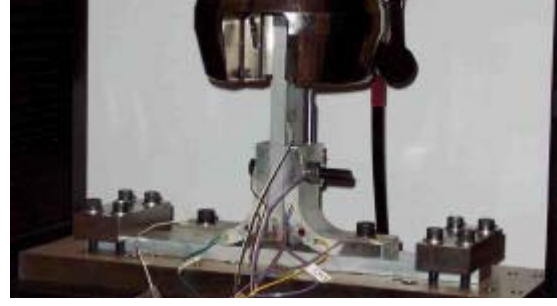
Figure 5: Direct tension loading of bolted aluminium T-joint (with strain gauges).
