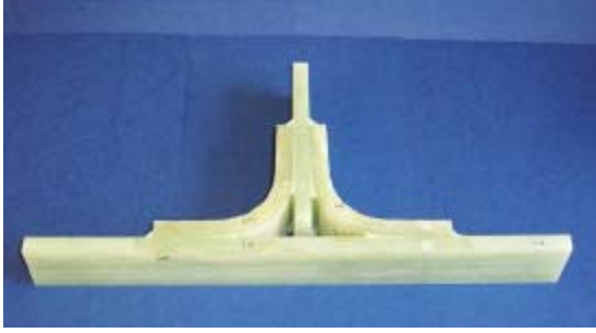
Figure 3: Bonded GRP T-joint.
