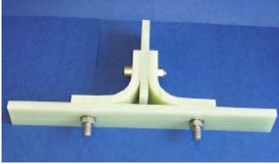
Figure 4: Bolted GRP T-joint.
