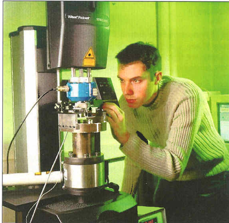
Figure 2. NPL 1.5 kN Hardness Machine.
