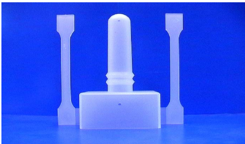
Figure 3 Moulded polypropylene part with left and right hand side tensile test bars (Wolfson Centre for Materials Processing, Brunel University).
