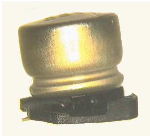
Figure 11 : 100 \mu F Electrolytic Capacitor after LF Reflow
