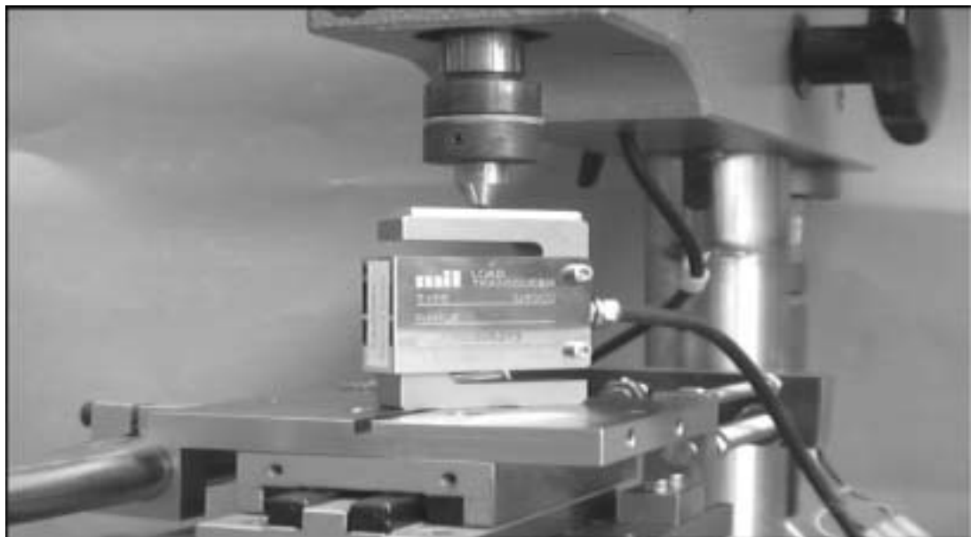
Figure A.1: Example of experimental setup for calibration of applied load
