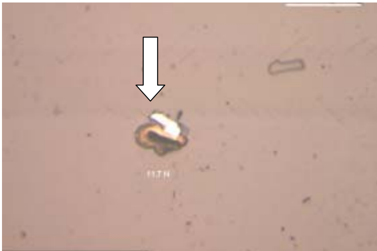
Figure B5: Micrograph of scratch track showing failure initiated at coating defect. The failure does not occur in a regular way and leads to a false value of critical load
