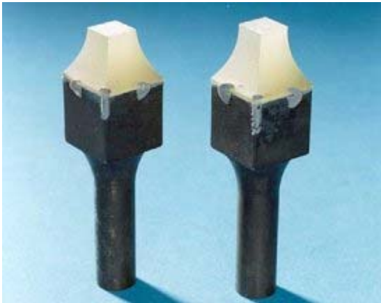
Figure 14: Failed RARDE tension specimen.
