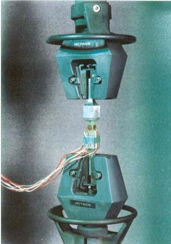
Figure 12: RARDE tension test (courtesy of DERA)
