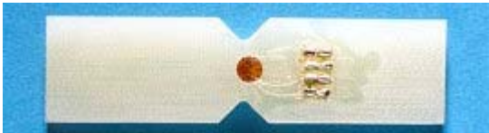
Figure 4: V-notched beam specimen. unidirectional glass fibre-reinforced laminate.
