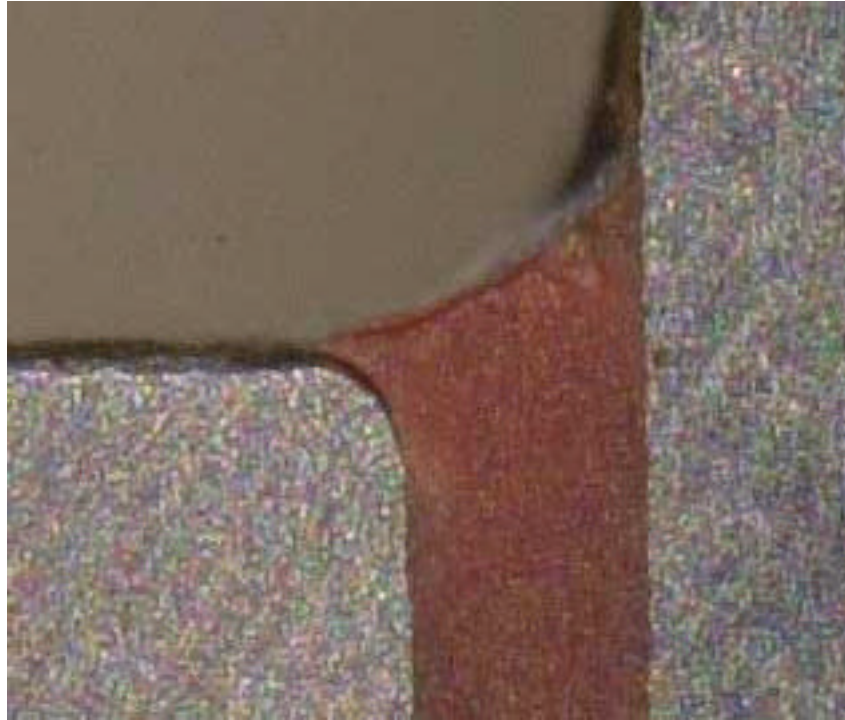
Figure 17. Photograph of a lap-joint specimen, after careful preparation of the side face, showing the interface crack prior to propagation through the thickness of the adhesive.
