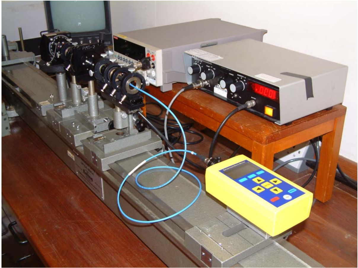
Figure 20. Stabilised source feeding optical fibre connected directly to PER meter
