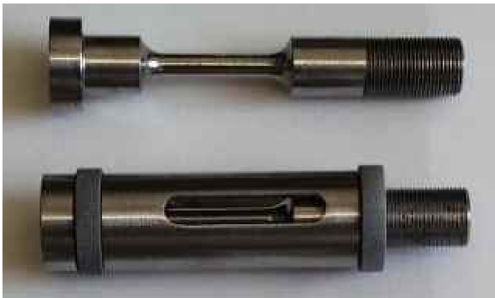
Figure 1. Photograph of the specimen and the loading frame for pitting and SCC tests.
