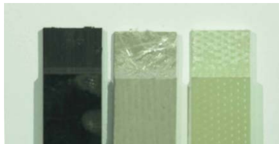
Figure 7 - Typical specimen failures in materials 1-3 respectively.
