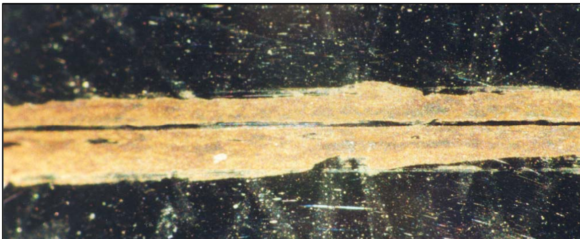
Figure 12 Wear scars from dry ball cratering sliding wear tests on TiN coated steel sample, a) crater on sample, b) track on ball.
