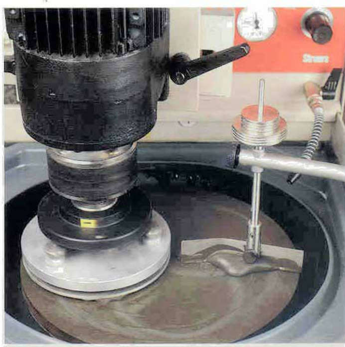
Figure 7, Struers micro wear test based on an automatic polishing system
