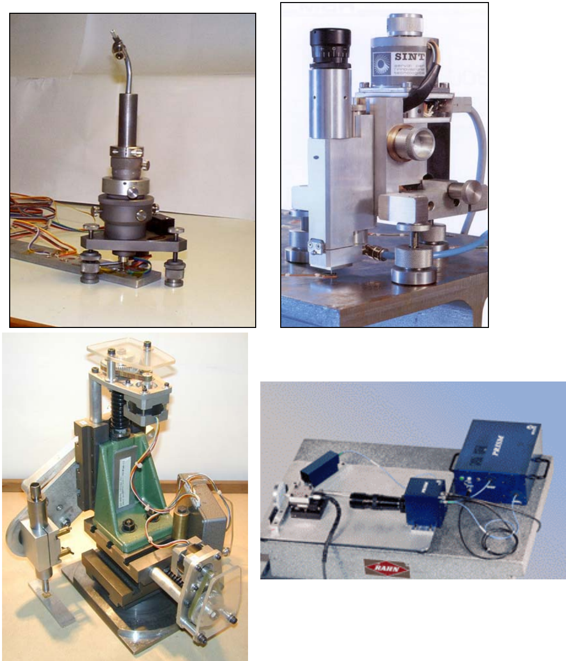
Figure 2: Typical commercial hole drilling rigs (clockwise from top left: Measurements Group, HBM, HYTEC Inc., Stresscraft Ltd)
