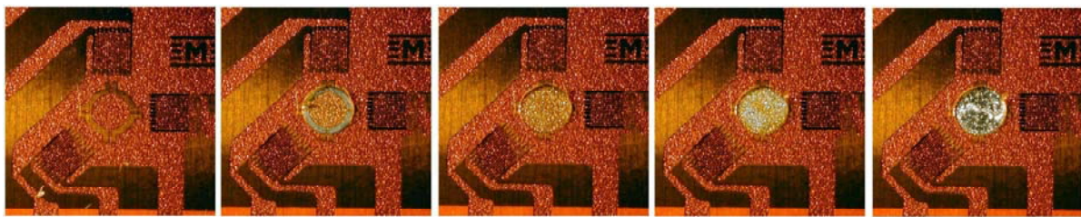
Figure 6: Stages of removing the gauge backing to reach the zero depth surface
