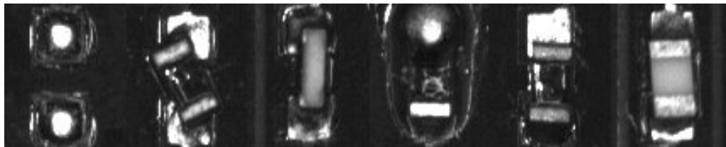
Figure 7 : Images of R0402 defects (from left to right - missing, misalignment, component on edge, excess, insufficient, inverted (source : Agilent))
