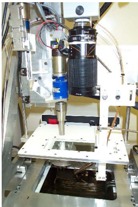
Figure 1: High rate extensional rheometer for testing molten polymers.
