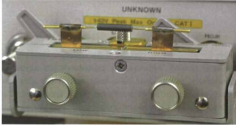
Figure 21: Piezoelectric sample placed between electrodes in the HP sample jig.
