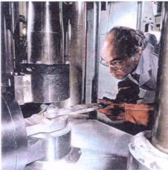
Hot billet being loaded into the "Grabber arm" of the large friction rig on the 700 ton press.
