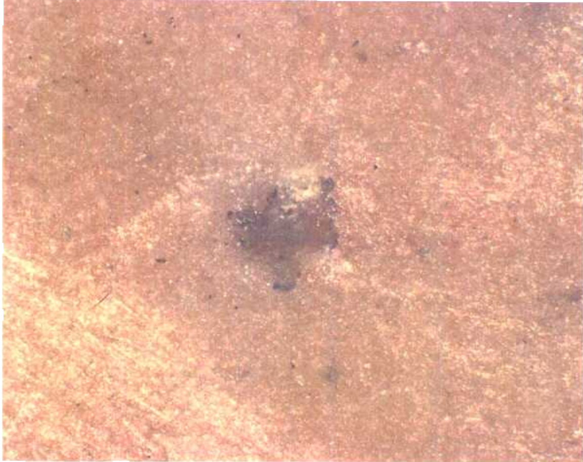
Figure 13 Pinhole in sample #35a probably caused by breakdown during poling
