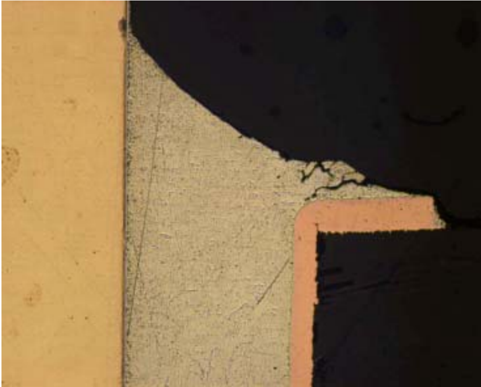
Fillet of SnAgCu / HASL after 2200 cycles
