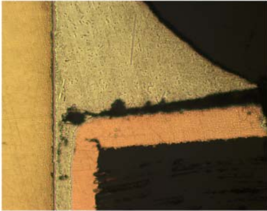
Fillet of SnAgCu / Cu after 1000 cycles
