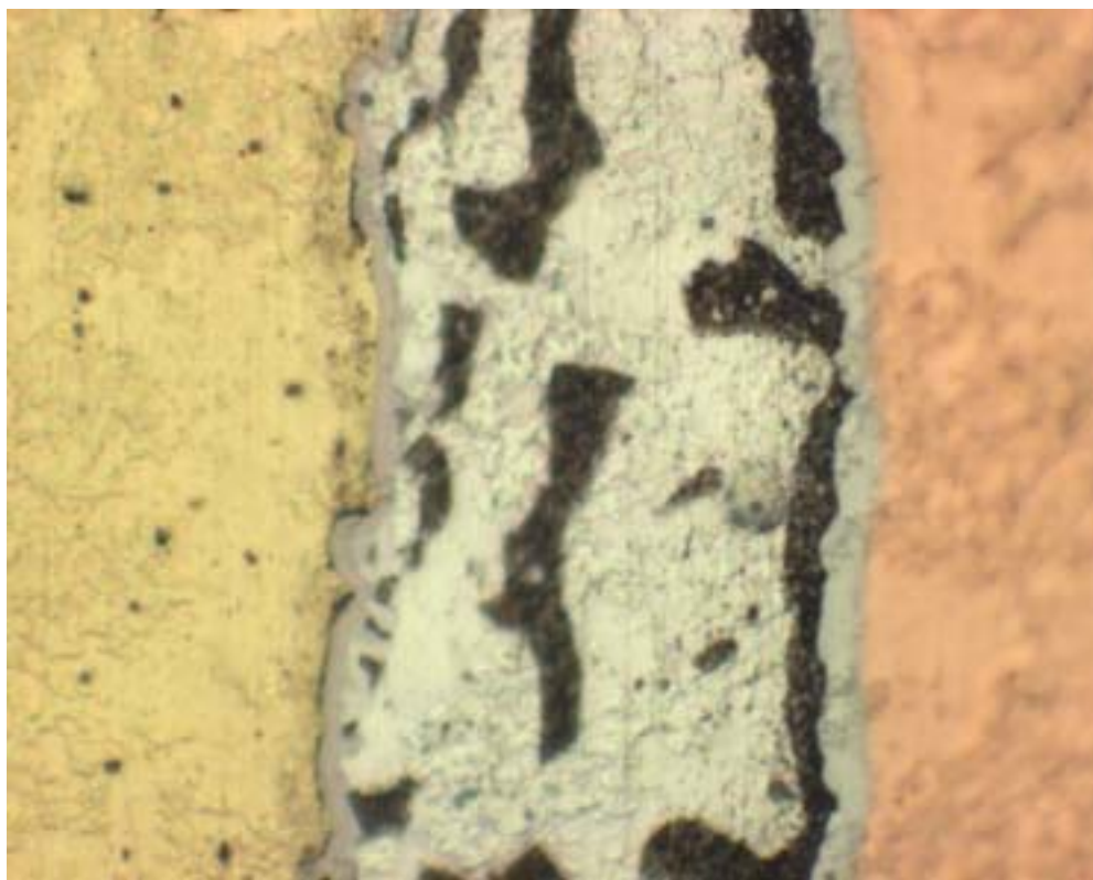
Intermetallic layer of SnPb / Cu after 2200 cycles
