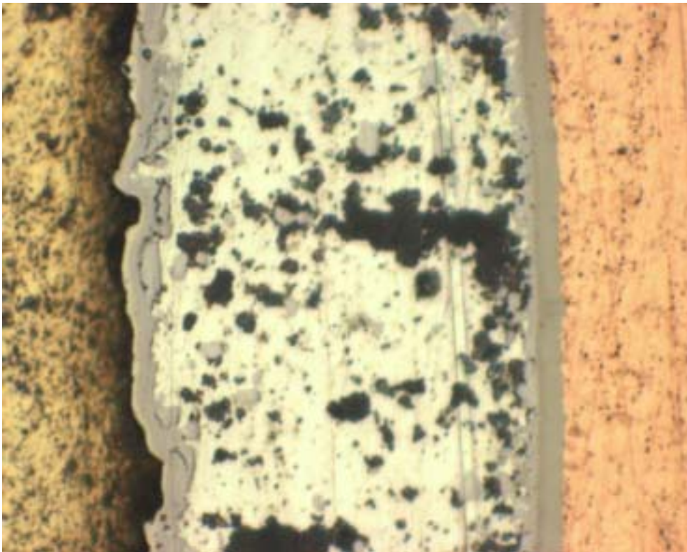
Intermetallic layer of SnAgBiCu / AuNi after 2200 cycles
