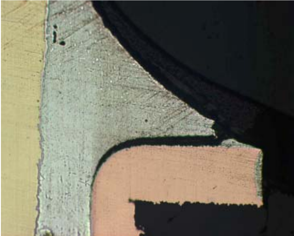
Fillet of SnAgBiCu / Cu after 400 cycles
