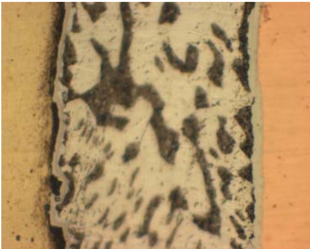
Intermetallic layer of SnPb / Sn after 2200 cycles
