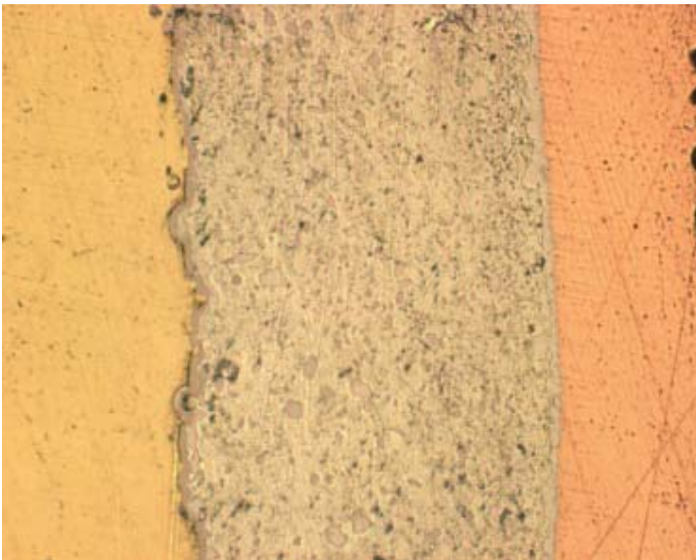
Intermetallic layer of SnAgCu / HASL after 2200 cycles
