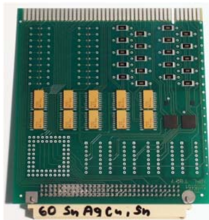
PCB with placed components for reflow soldering
