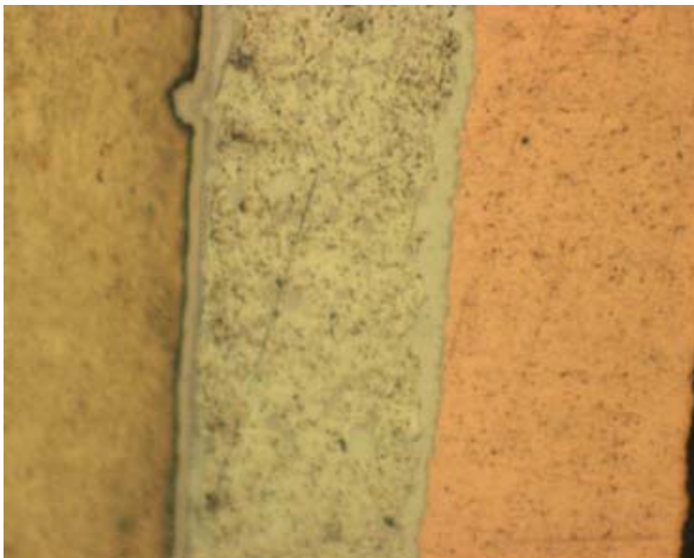
Intermetallic layer of SnAgCu / Cu after 1000 cycles
