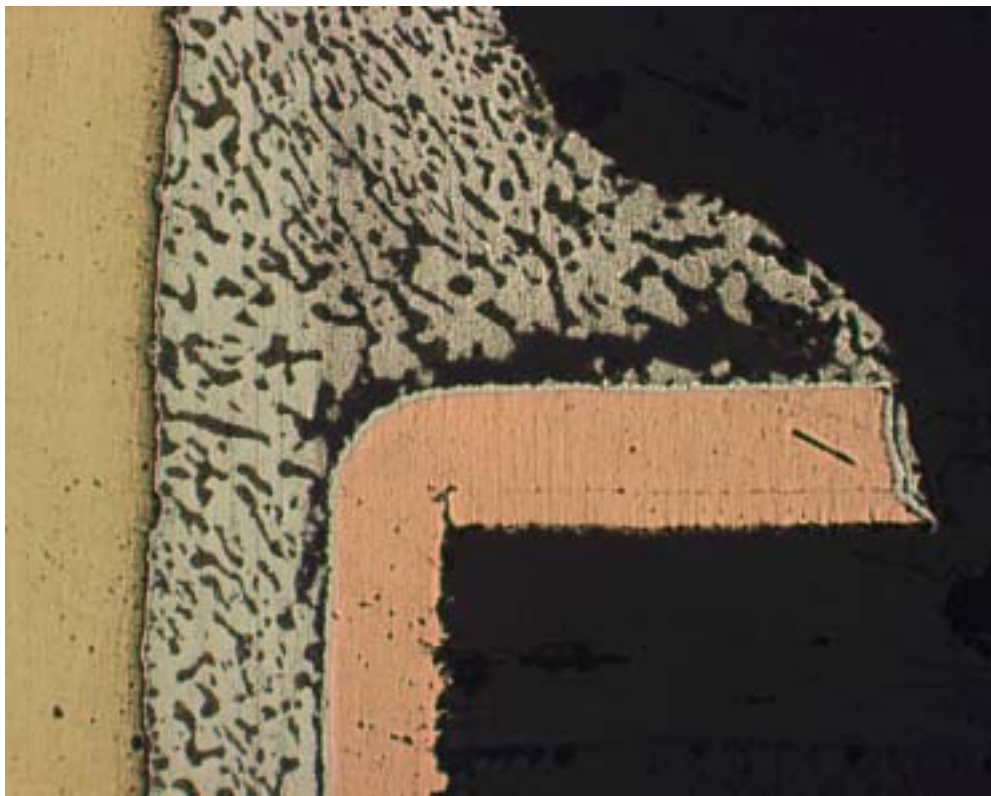
Fillet of SnPb / Cu after 2200 cycles
