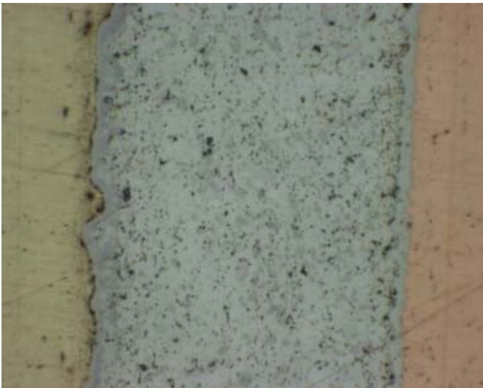
Intermetallic layer of SnAgBiCu / Cu after 400 cycles
