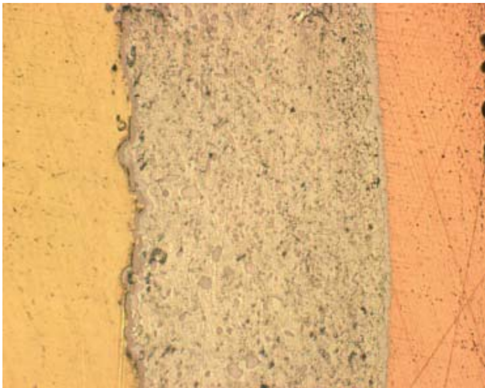
Intermetallic layer of SnAgBiCu / HASL after 1000 cycles
