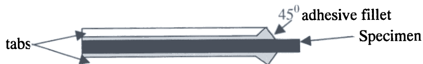
Figure 9 Design of end tabs for compression specimens.
