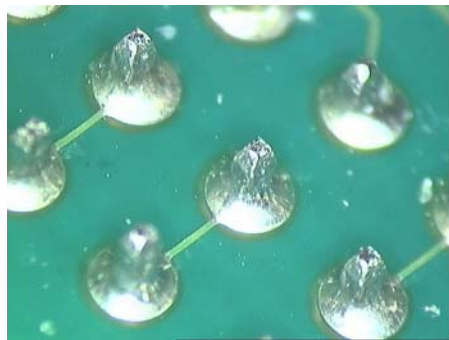
Figure 22: TH joint using 100% SnPb solder
