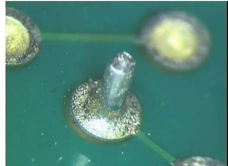
Figure 19: TH joint using 75%/25% SnAgCu/SnPb solder
