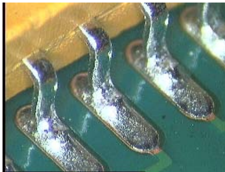
Figure 47: SOIC joint using 100% SnAgCuBi solder
