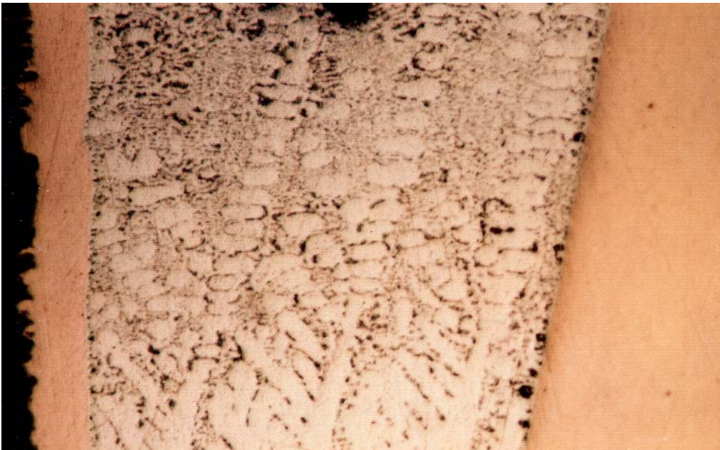
Figure 70. SnAgBiCu/ 75% SnPb TH-Resistor joint (x390).
