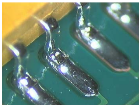
Figure 27: SOIC joint using 100% SnPb solder
