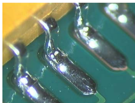
Figure 17: SOIC joint using 100% SnPb solder
