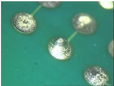
Figure 20: TH joint using 50%/50% SnAgCu/SnPb solder
