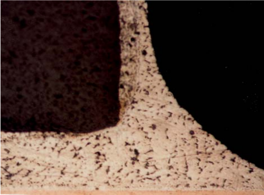
Figure 81. SnPbAg/ 75%SnAgCu 2512 Resistor joint. (x390)
