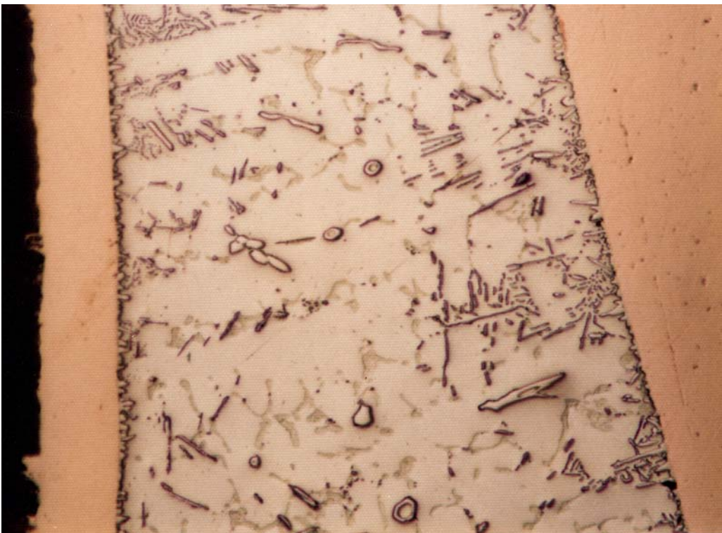
Figure 68. SnAgBiCu/ 25% SnPb TH-Resistor joint (x440).
