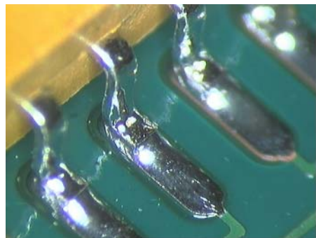
Figure 37: SOIC joint using 100% SnPb solder
