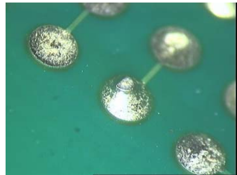
Figure 21: TH joint using 25%/75% SnAgCu/SnPb solder
