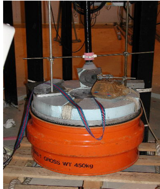
Figure 2-3: Apparatus for removing or storing the source in the lead pot
