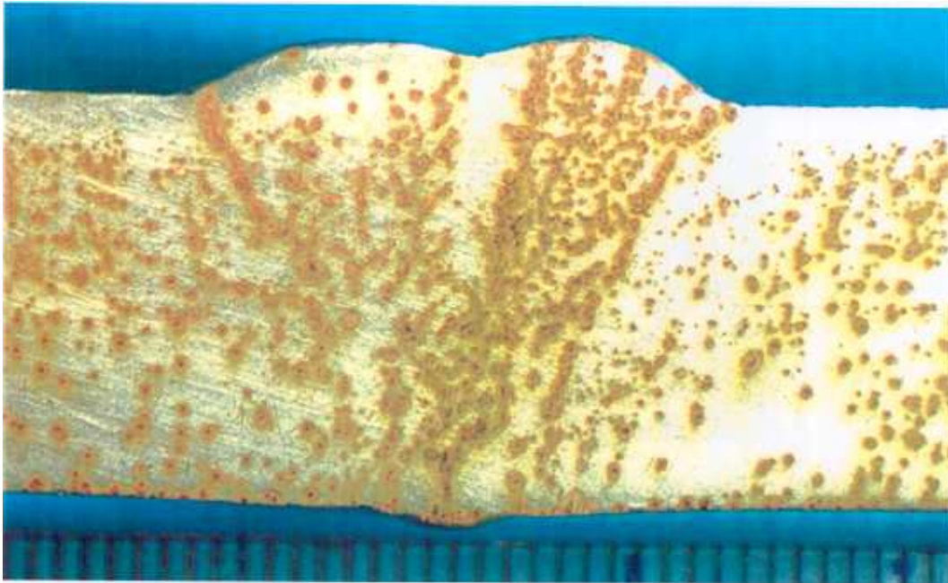
Figure 5. Visual appearance of weld Y after exposure to distilled water for 60 minutes showing corrosion at discrete anodes.
