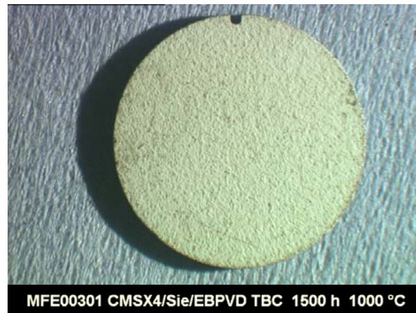
Figure 15 Optical micrograph of a typical test sample for the piezospectroscopic investigation showing relocation notch.
