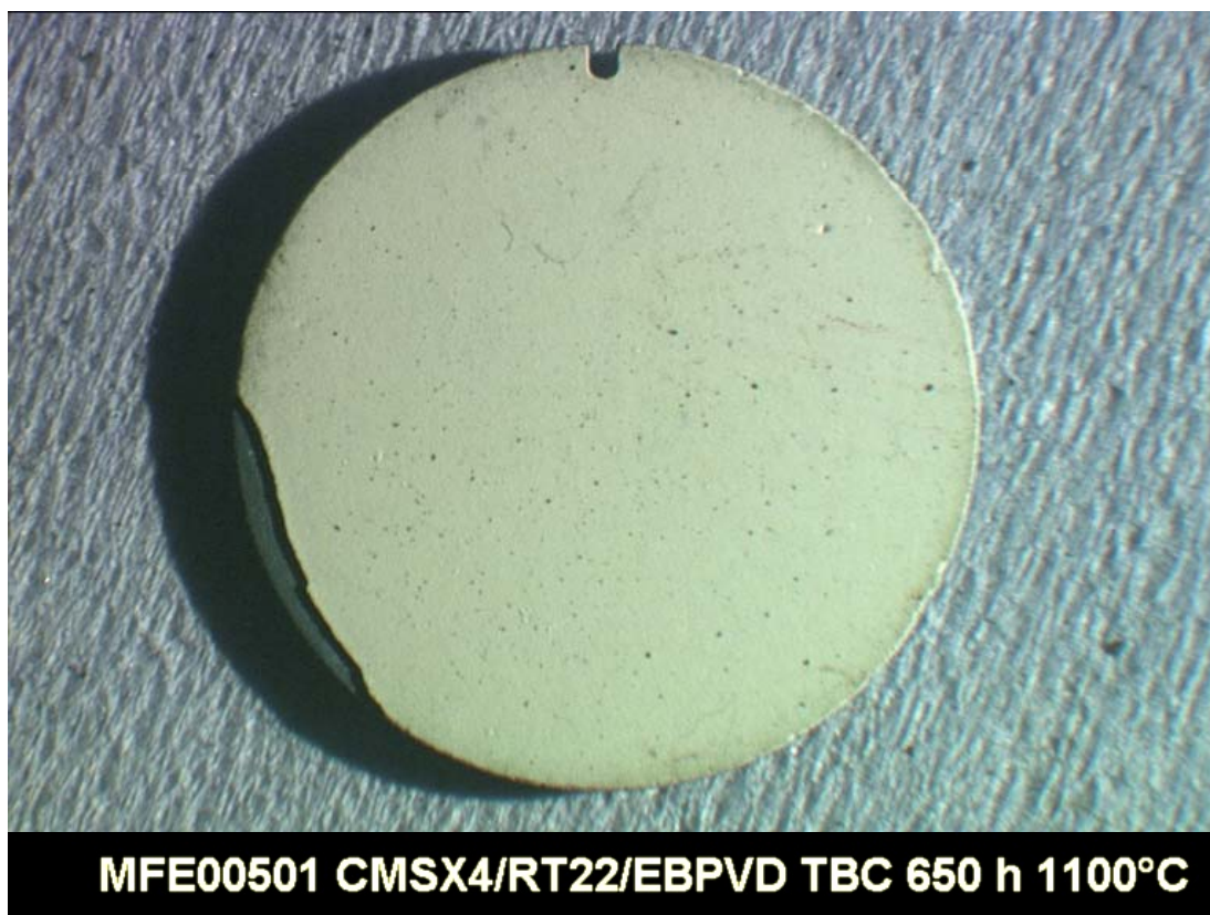
Figure 31 Optical micrograph of CMSX4/RT22/EB-PVD aged for 650 h at 1100 °C with the slow cool cycle
