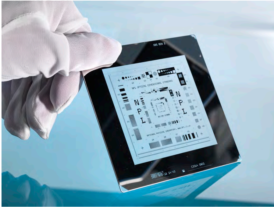
Figure 31: NPL's ODS, which contains patterns specifically designed to identify and quantify errors in a range of optical systems.
