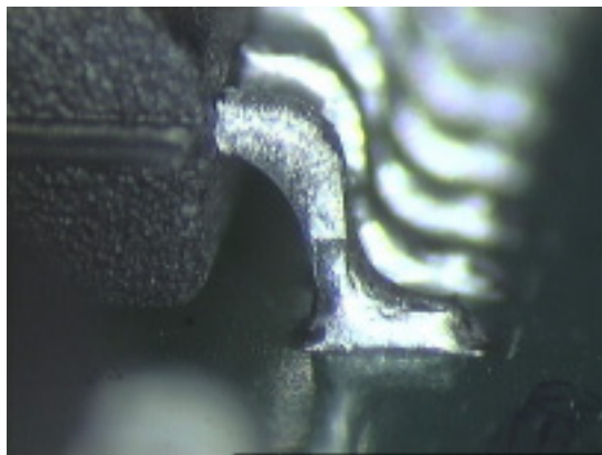
Figure 69: Example of SnAg1 solder joint where plating has reflowed
