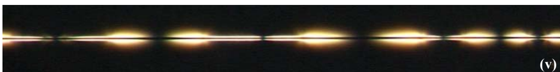
Appendix F1 – Images detailing damage progression in a single break in a standard carbon specimen under full extinction with increasing stress; (i) ~45MPa, (ii) ~52MPa, (iii) ~57MPa, (iv) ~60MPa and (v) ~66MPa.
