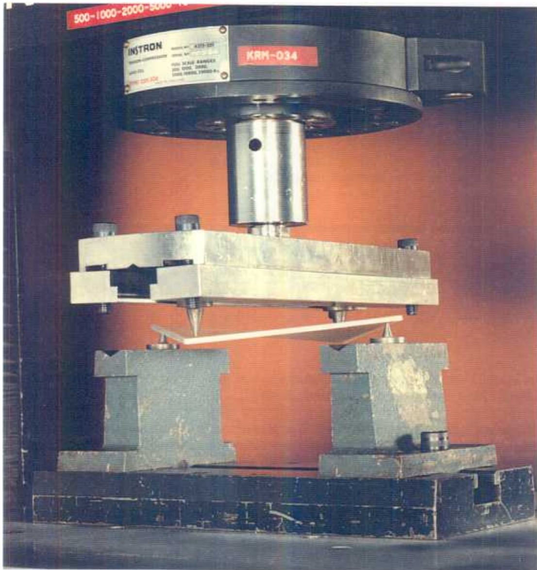
Figure 2 Plate under load on universal test machine.
