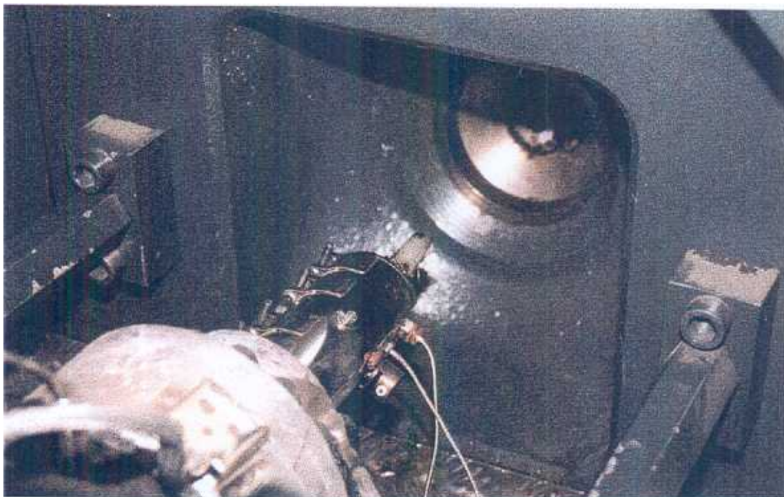
Figure 9. Schematic diagram of the nozzle set-up and a picture of the nozzle fitted on an injection moulding machine.
