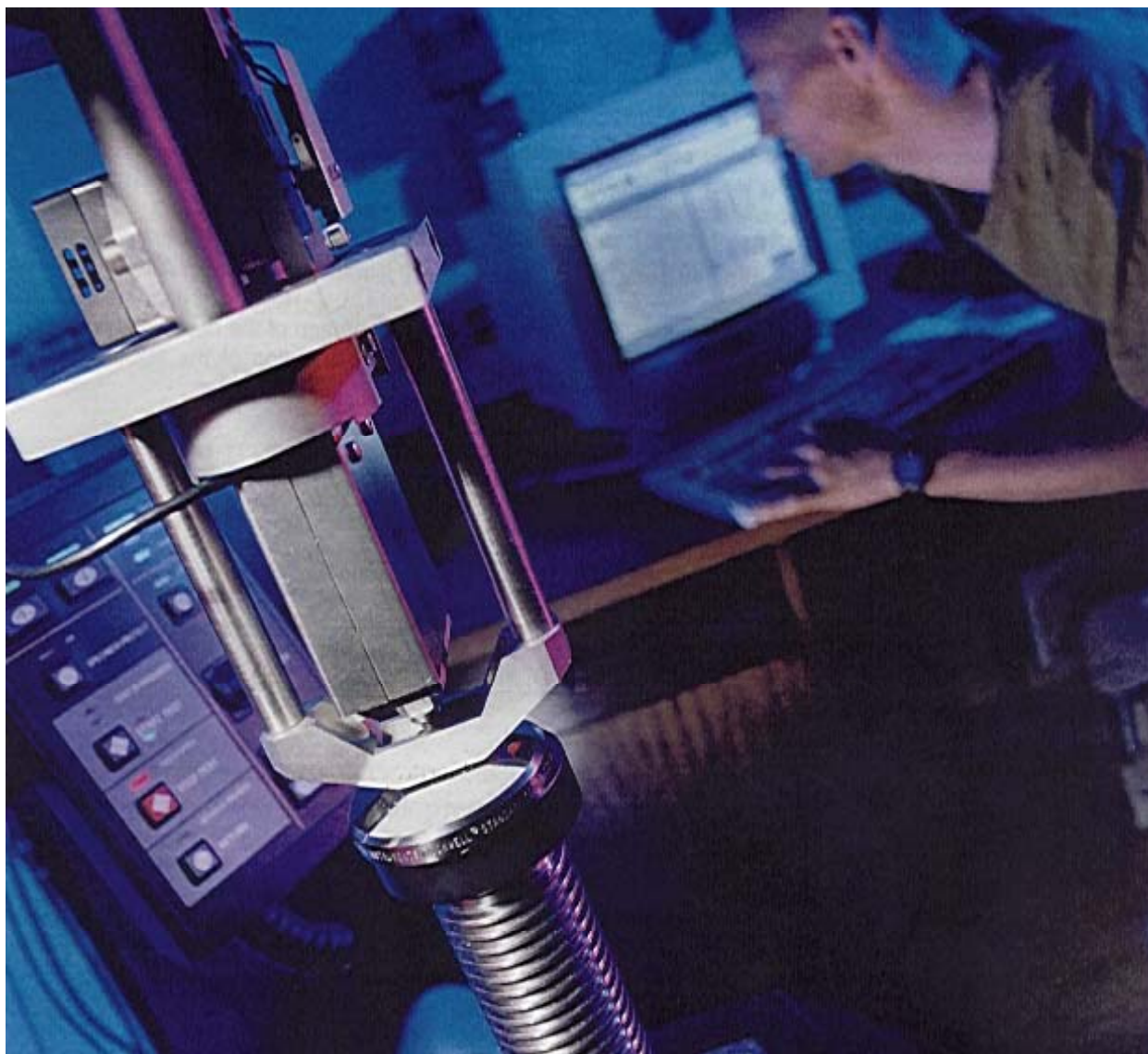
Figure 1. Machine 1, applies forces from 30 N to 1 500 N.
