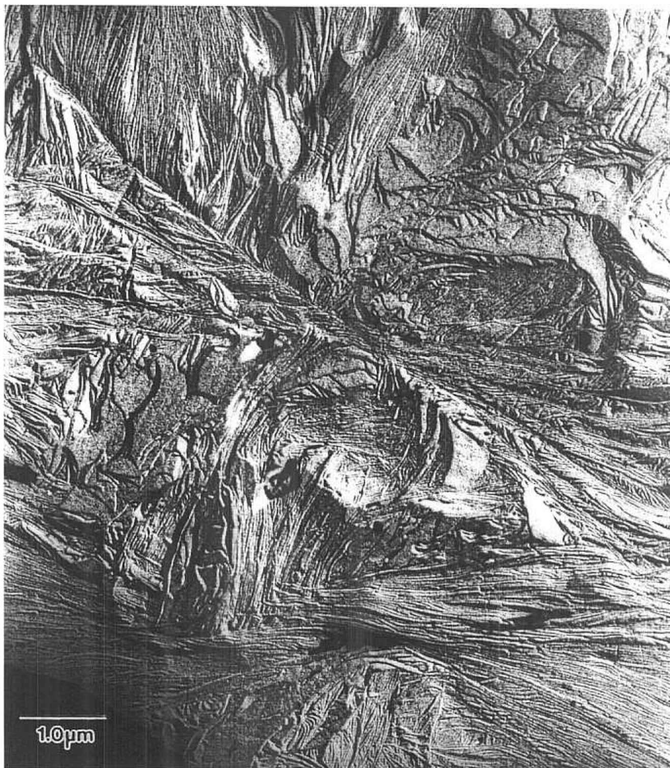
Fig. 17 TEM carbon replica of dry permanganically etched yellow 93 crystallized under controlled cooling conditions of 10K/min from 430K. Region highlighted is of a spherulitic sheaf (centre) with characteristic dominant-subsidary structures and areas of spherulitic impingement on either side.
