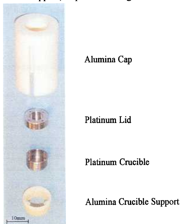
Figure 5 Picture of slag cell (lid and crucible), holder and cap.
