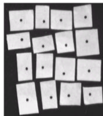
Figure 7: Grid of dots used to measure the strain in a biaxial specimen
