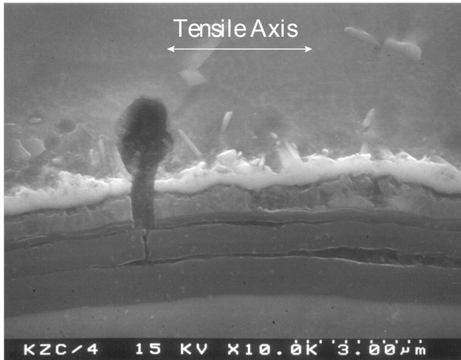
Figure 8: 90° MMC After Cycling to 700°C and Tensile Test
