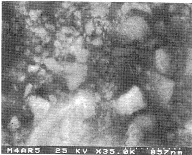
Figure 7, Worn surface of hardmetal tested in ASTM B611 test showing fragmentation of WC grains.
