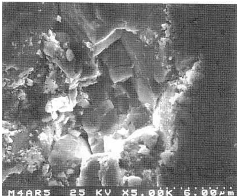
Figure 7, Worn surface of hardmetal tested in ASTM B611 test showing fragmentation of WC grains.
