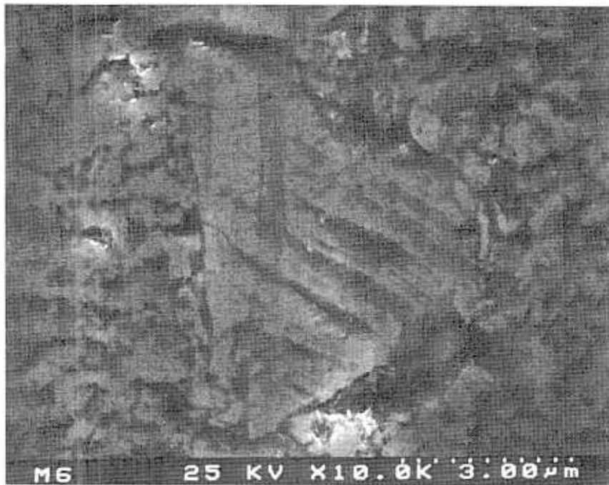
Figure 9, Single large WC grain damaged in ASTM B611 test on hardmetal sample.
