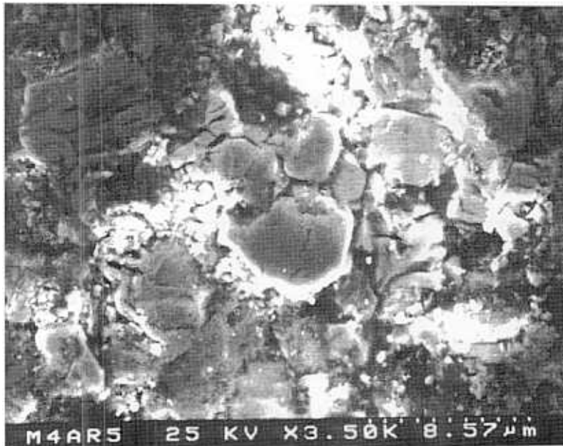
Figure 6, Fragmentation of WC grains on hardmetal surface worn in an ASTM B611 test.
