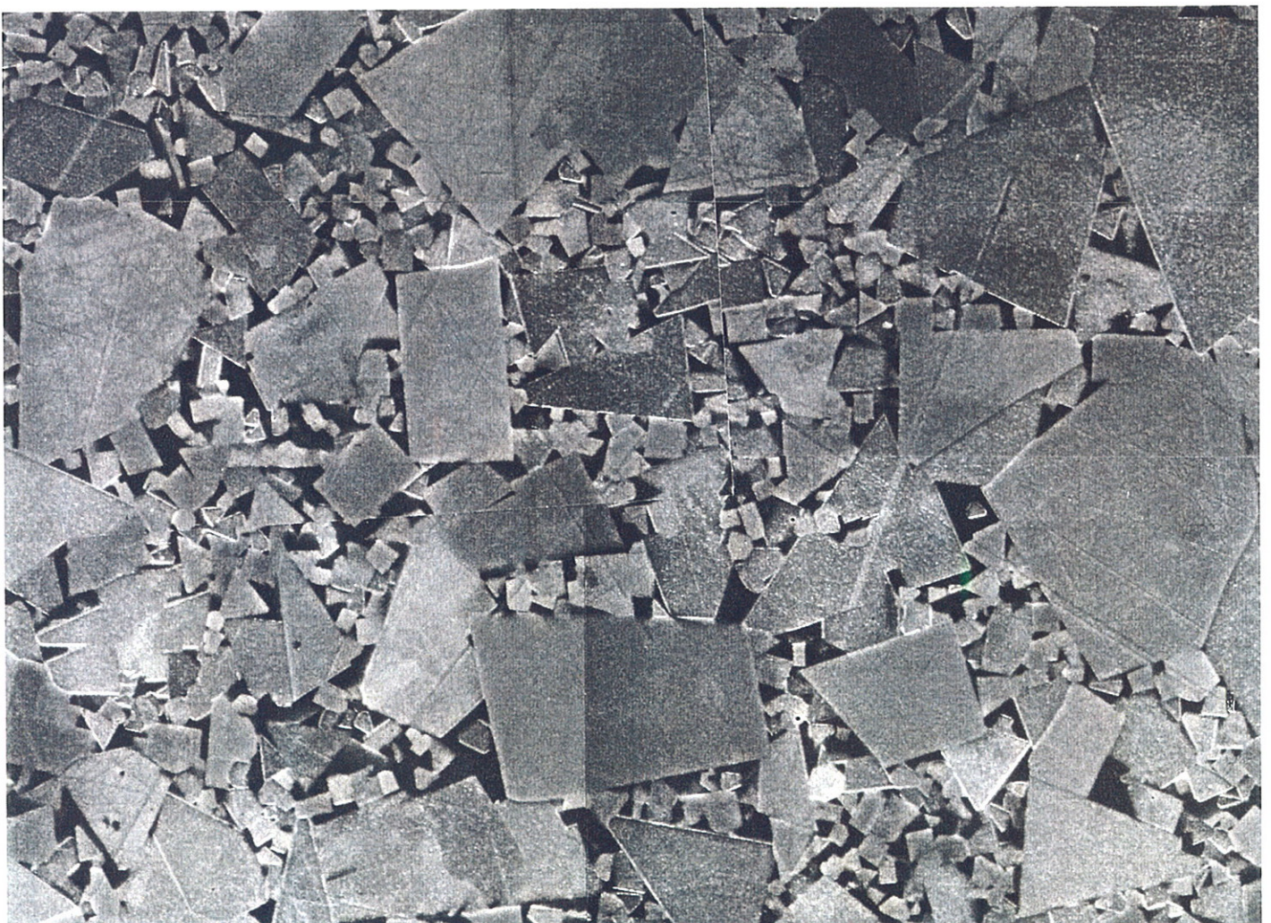
Fig 2 Micrographs of conventional WC/Co (D1) and wide grain size distribution WC/Co (F12)
